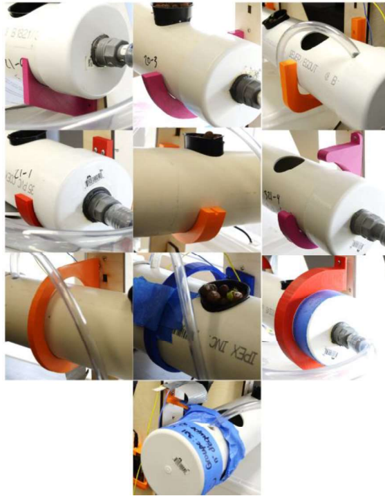
Figure 5. Main tank support bracket variations
