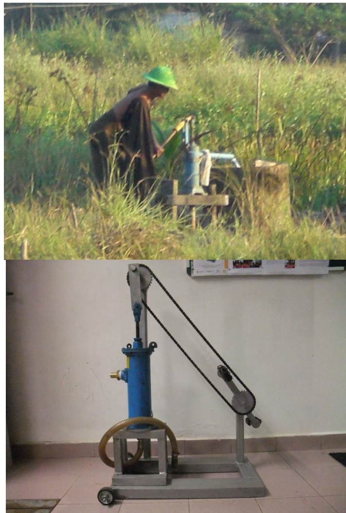
Figure 4: (Top) A Myanmar man in a village in Yangon using a hand pump to draw water from a well. (Bottom) A modified hand pump designed by the students that uses paddling action to provide physical force to move water.
